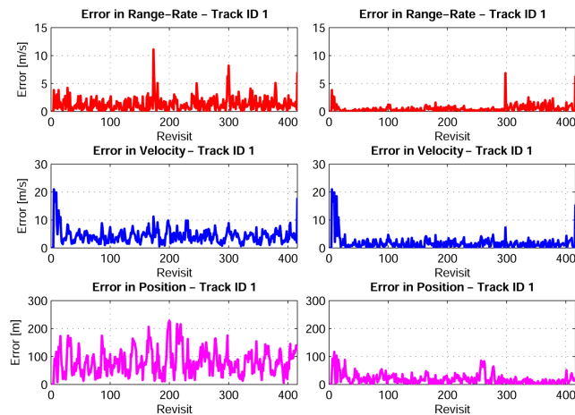
Figure 5: Track errors wrt. ground truth information for the single target scenario, see Fig. 4, without (left column) and with (right column) exploitation of road-map information.
